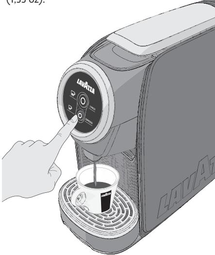
**i** The switch-on/supply button will light up to a blinking white light when the product is being supplied.
