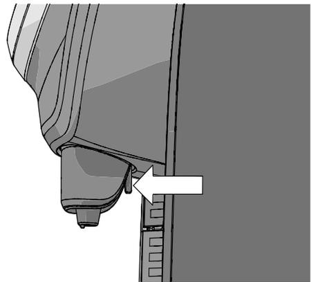
**6** Insert the the spouts into the machine, paying attention to the click that indicates its proper functioning.
