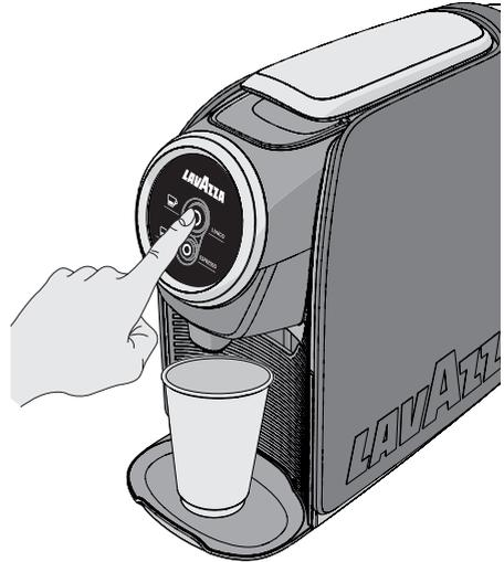
**6** For a new supply cycle, wait for supply buttons and multifunction button turning on with steady white light.
