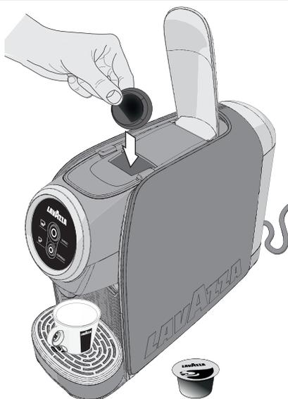
**4** Lower the capsule loading lever to close the pod fitting compartment.
