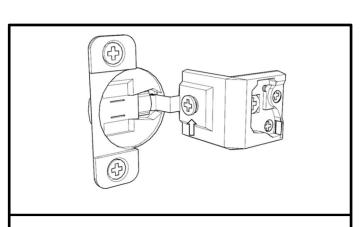
If the door is not level when it is installed, the customer will need to turn the screw clockwise to extend the hinge or counterclockwise to shorten the hinge.
