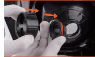
Fig. 3: Assemble the retainer holder with the bulb retainer together, and then insert them into the assembly.
