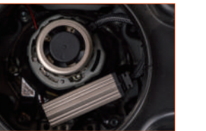
Fig. 4: Sort and fix the wiring harness with Zip Ties or Double-side Tape. You can also insert the drive into assembly.
