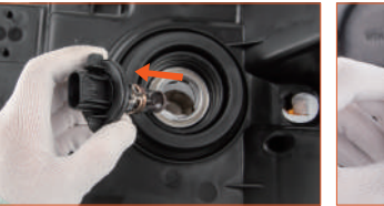
Fig. 1: Remove the OE halogen bulb
