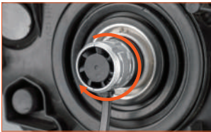
Fig. 3: Insert the lamps , turn them clockwise, then clamp tightly.
