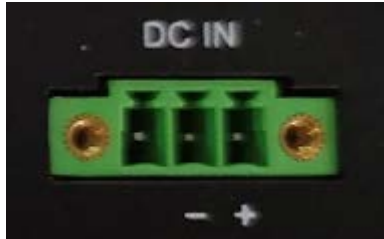
Figure 5-1-1 DC24V power input connector
