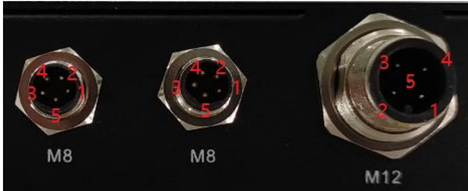
Figure 5-2-1 Power Output & CAN Interface
