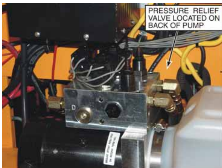
Figure 4-6. Pressure Relief Valve Adjustment
