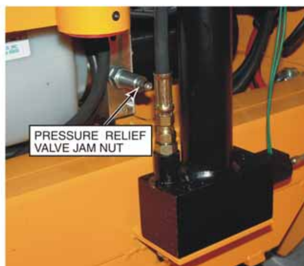
Figure 4-6. Pressure Relief Valve Adjustment
