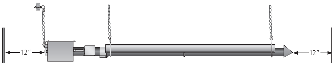
Figure 2.27 • Minimum end clearance for unvented heater
