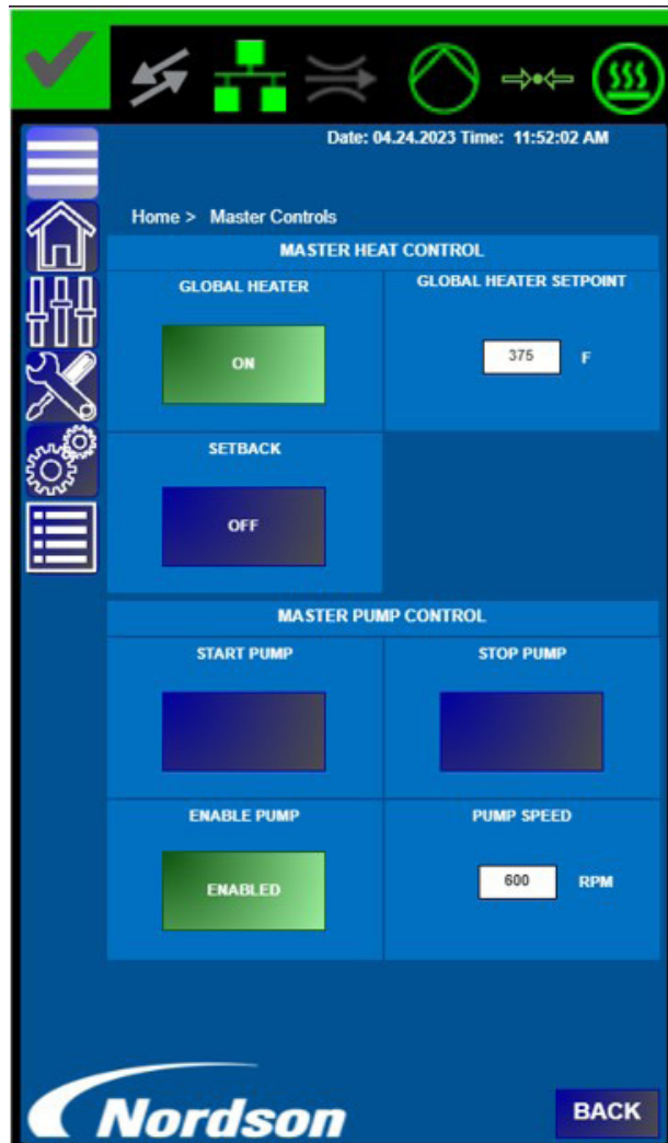
Figure 4-6: Master Controls screen
