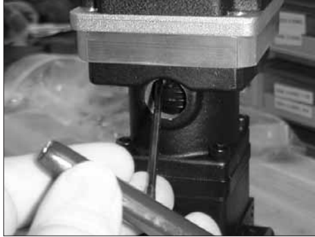
Figure 7-49 Removing the motor shaft set screw
