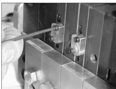
Figure 7-17 Removing a miniature pressure transducer from a pump
