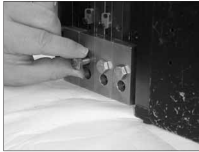
Figure 7-32 Installing a pump clamp
