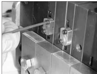
Figure 7-110 Removing a pressure transducer plug (pump location shown)
