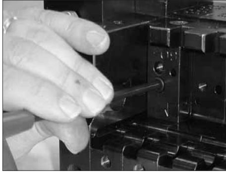
Figure 7-28 Installing an adhesive diverter plate
