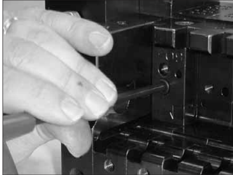
Figure 7-72 Installing an adhesive diverter plate
