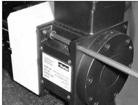
Figure 7-40 Installing the reducer/motor assembly
