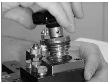
Figure 5-1 Removing the filter knob
