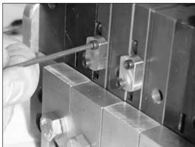
Figure 7-46 Removing pump pressure transducer plugs
