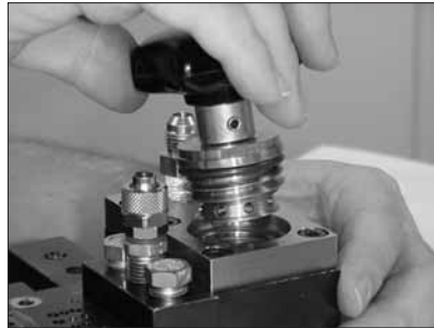
Figure 7-55 Removing the filter knob and filter basket
