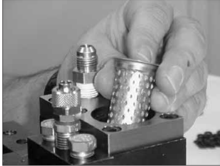
Figure 5-2 Replacing the filter basket
