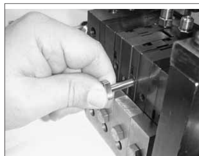
Figure 7-17 Removing a miniature pressure transducer from a pump
