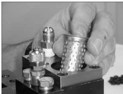
Figure 7-70 Installing the filter basket and knob
