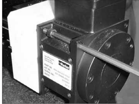
Figure 7-21 Removing the reducer/motor assembly
