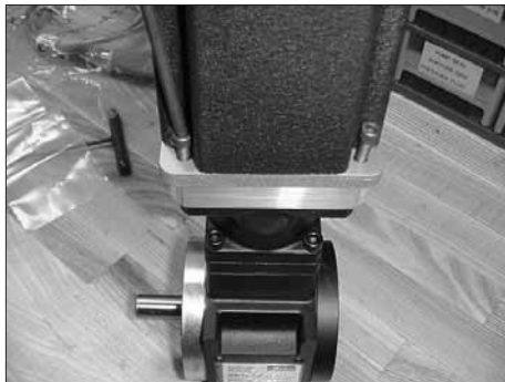
Figure 7-50 Removing the motor from the reducer
