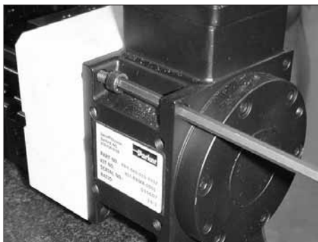
Figure 7-95 Removing the reducer/motor assembly
