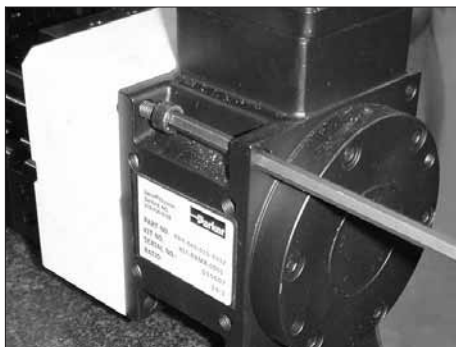
Figure 7-47 Removing the reducer/motor assembly
