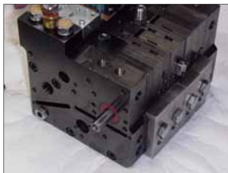
Figure 7-101 Applicator ready for drive assembly installation on the opposite side
