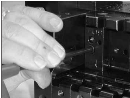
Figure 7-54 Removing adhesive diverter plates
