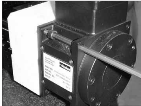
Figure 7-105 Installing the reducer/motor assembly
