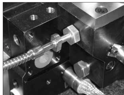
Figure 7-16 Removing a miniature pressure transducer from the filter block
