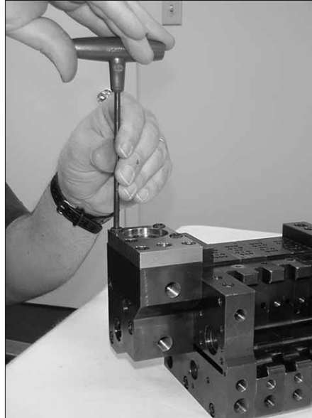
Figure 7-57 Removing the filter block cap
