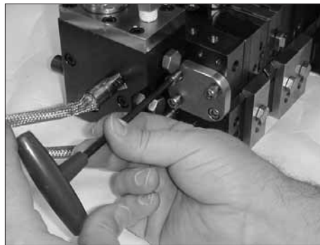
Figure 7-106 Removing the pump shaft end cap
