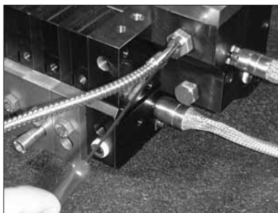
Figure 7-16 Removing a miniature pressure transducer from the filter block
