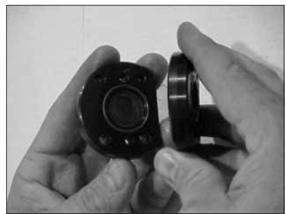
Figure 7-103 Replacing the pump packing O-ring and spring seal
