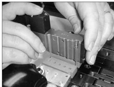
Figure 7-86 Installing solenoid valves
