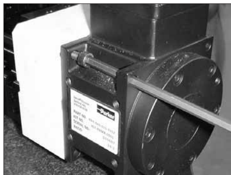
Figure 7-88 Installing the reducer/motor assembly
