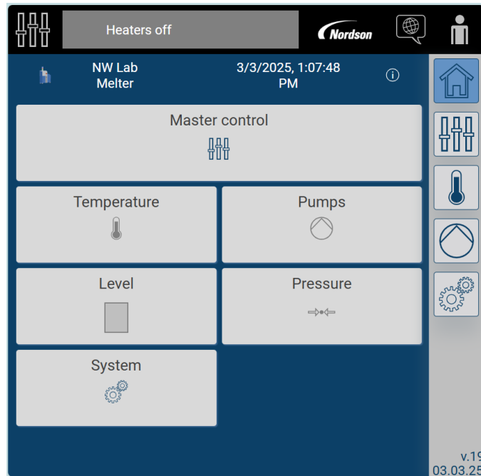
Figure 2-9 Home screen on control panel
