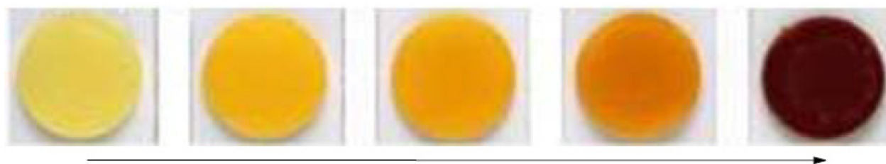
Figure 6-3 Aging/coking of hot melt adhesives when heated too long
