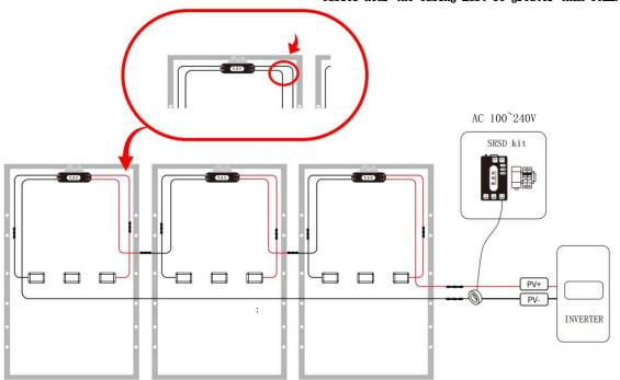
2 The following diagram shows the networking scenario of the optimizer and the intelligent acquisition gateway:
