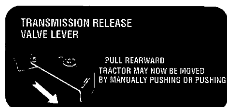
Decal - Hydro Release Valve Part No. 1706916
