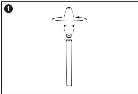
2. Place the wire at the notch of the stake, and screw the stake clockwise onto the pole.
