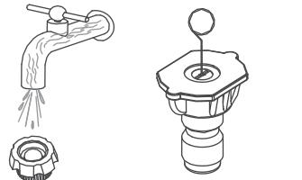
2. Using the nozzle tip cleaner provided ( or an unfold paper clip ), insert the wire into the nozzle hole and move back and forth until debris is dislodged. Back flush water through the nozzles using garden hose and highest pressure available (either standard water nozzle or use your thumb over the nozzle to create water pressure for back flush )
