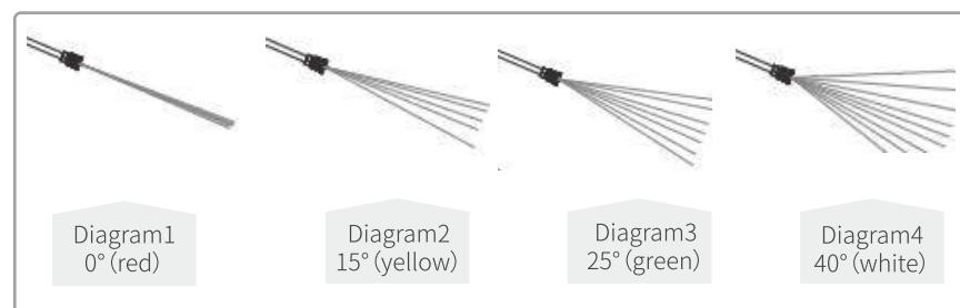
0°nozzle-red : This type of nozzle produces a vertical, stratified, high-pressure jet for surface cleaning with particularly severe dirt.
