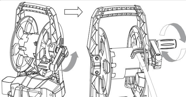
When not in use, insert the quick-connect end of the high pressure hose into the hook of the reel, turn the hose reel handle counterclockwise, and reel the hose onto the reel.
