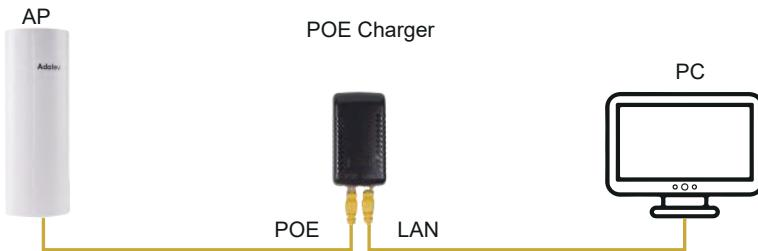
Refer to the figure left to connect the CPE to the computer through a POE adapter and an Ethernet cable.
