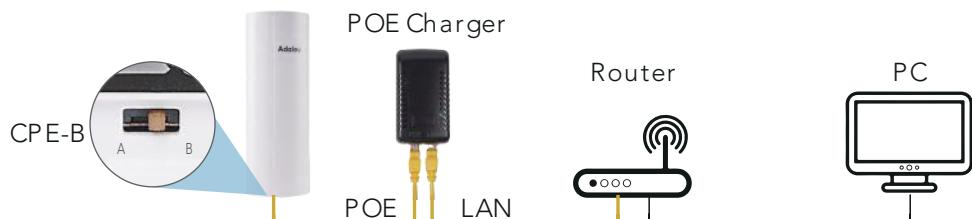
Step 1: The POE port of the POE adapter connect to the POE/LAN port of slave bridge through an Ethernet cable
