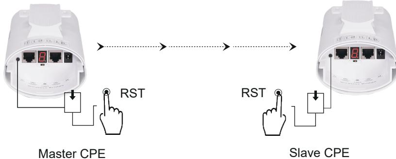
3. Wait them for pairing. When the signal light on the side turns on, it means the pairing is successful;
