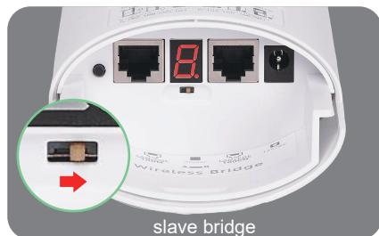
2. Short press the reset button to change the channel from 0-9, A-F, the LED indicator will display the numeric to show what channel it is, please keep the master and slaves bridges in the same channel.
