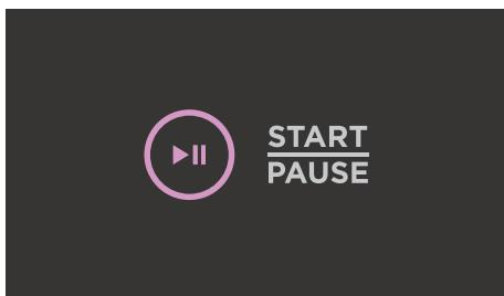
**►II** will illuminate when the **LID LOCK** is active. To unlock the lid at any time during the cycle, press **►II**. In some circumstances, there may be a delay before the lid can be opened, for safety reasons.
