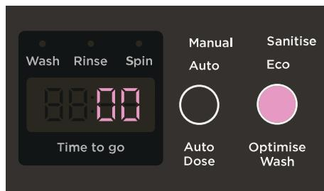
Press **OPTIMISE WASH** until is displayed on the screen. Your washer will now adjust the cold temperature to approximately 20°C.
