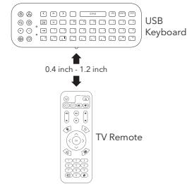
3. Press and release the button you wish to program on the device. The red LED will blink quickly and then turn OFF when the button has been programmed. Repeat these steps to program the other buttons.
