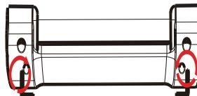
If deviating turns to right, then turn the left screw in counter-clockwise direction,turn the right screw in clockwise direction.
