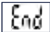
Repair process ended
