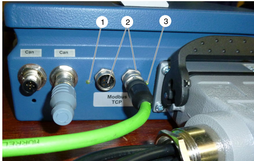
Fig. 3 Example: OptiStroke with Modbus interface
