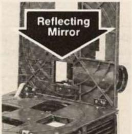
To install a replacement Quartzline lamp (ASA Code ELH), run the projector with the switch in the FAN position until the old lamp has cooled THOROUGHLY. Turn the switch OFF, UNPLUG THE POWER CORD, and turn the projector on its side or back.
