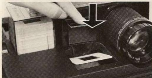
**NOTE:** If a slide is incorrectly positioned in the **Previewer**, push down on the **Slide Ejector** to tilt the slide up. Then remove, reposition, and replace slide in **Previewer** before pressing the **Slide Advance**. If a slide is incorrectly positioned when projected, move **Forward/Recall Switch** to **RECALL**, press **Slide Advance**, then use **Slide Ejector** to remove / reposition / replace slide in the **Previewer**. Return switch to FORWARD position and resume show.
