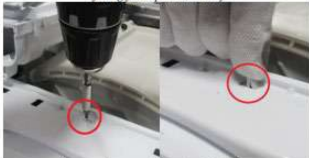
Remove the screw fixing twinjet elbow.
