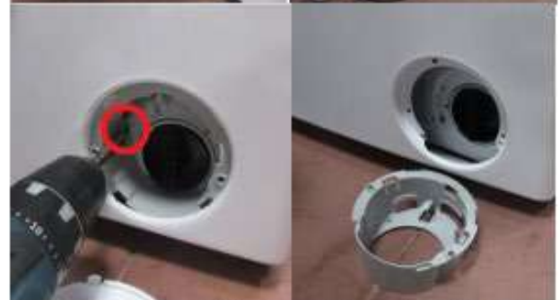
Remove the screw and plastic part located under the pump cover
