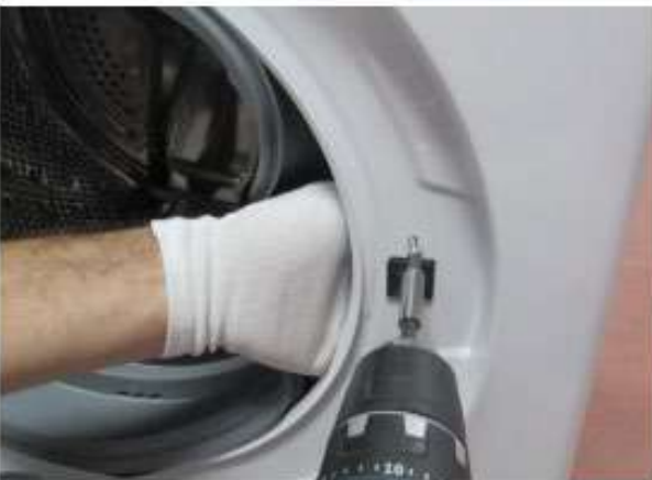
Tighten the door lock screw
