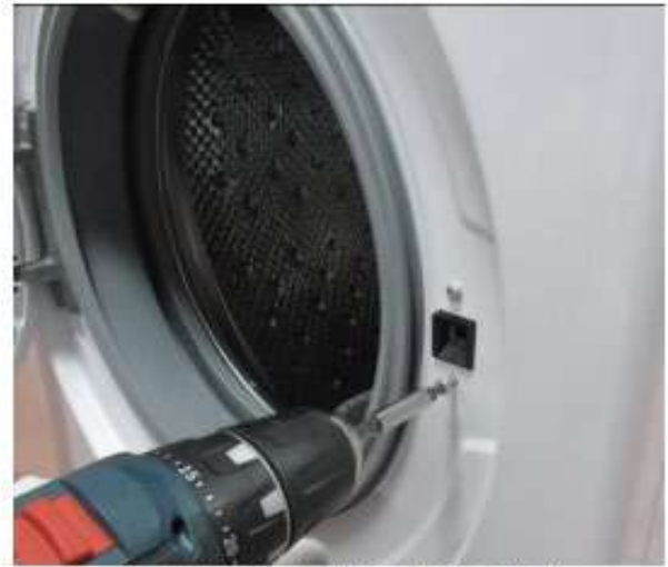
Remove the screws fixing the door lock.
