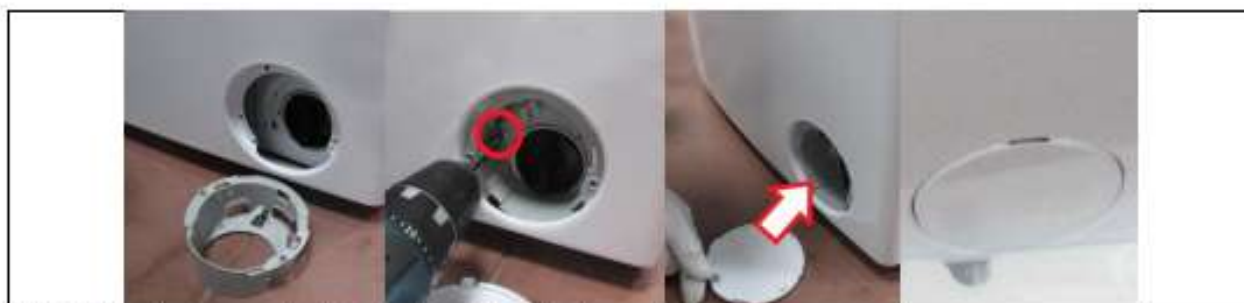
3.7. Tighten the screw and plastic part located under the pump cover
