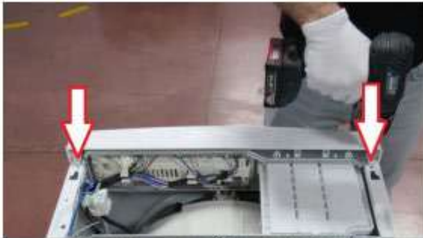
Remove two screws fixing control panel.
