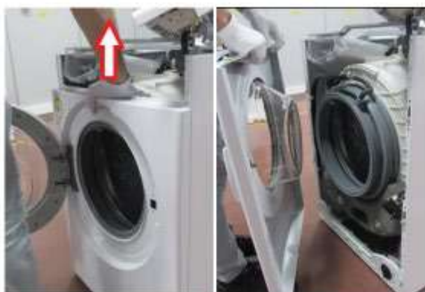
Pull up and remove the front panel.
