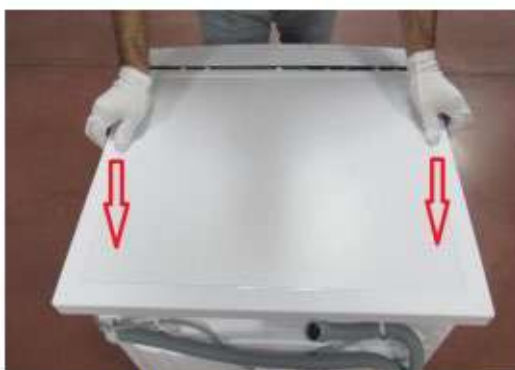
Push the top-plate back and pull it up.
