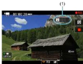
As the internal temperature rises, the level on the indicator extends to the right. How fast the level increases will depend on shooting conditions. Levels 1–7 are marked in white, but once the temperature reaches level 8, the color changes.
