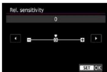
For faster AF point positioning, set toward the positive end, and for slower positioning, set toward the negative end.
