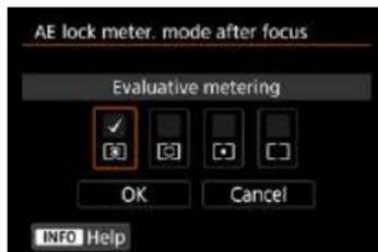
For each metering mode, you can specify whether to lock the exposure (AE lock) once subjects are in focus with One-Shot AF. The exposure will be locked while you keep pressing the shutter button halfway. Select metering modes for AE lock and add a checkmark [✓]. Select [OK] to register the setting.
