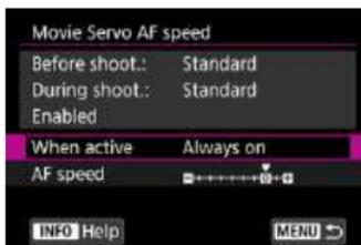
You can set **[Always on]** to have the AF speed take effect at all times for movie recording (before and during movie recording) or set **[During shooting]** to have the AF speed take effect only during movie recording.
