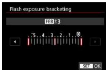
Speedlites equipped with flash exposure bracketing (FEB) can change the external flash output automatically as three shots are taken at once.
