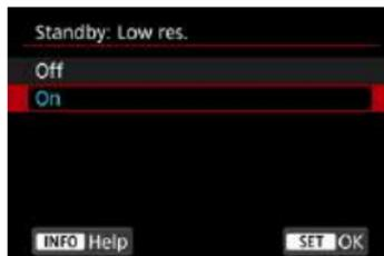
Set to **[On]** to conserve battery power and control the rise of internal camera temperature during standby.
