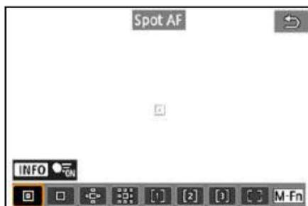
The camera focuses in a narrower area than 1-point AF.
