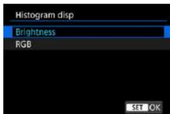
The histograms show signal levels across the tonal range. Brightness display (for checking the general exposure level and overall gradation) and RGB display (for checking saturation and gradation of red, green, and blue) are available. You can switch the histogram displayed by pressing the <INFO> button when [INFO] is displayed in the lower left of the [▶]: **Playback information display** screen.
