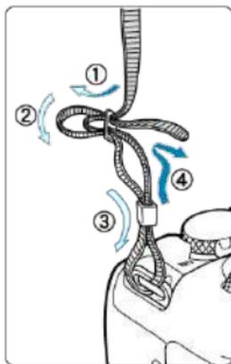
Pass the end of the strap through the strap mount from the bottom, then pass it through the strap buckle as shown. Pull the strap to take up any slack and make sure the strap will not loosen from the buckle.
