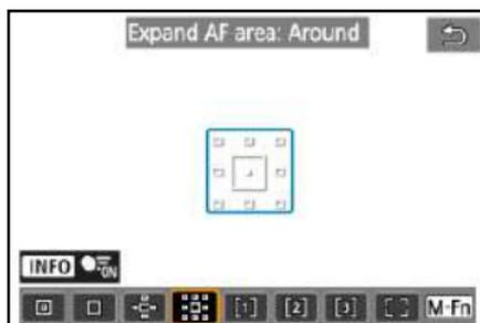
Focuses using one AF point (☐) and the surrounding AF area outlined here in blue, which makes it easier to focus on moving subjects than with Expand AF area: ☒.
