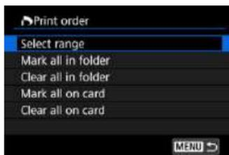
Select **[Select range]** in **[Multiple]**. Selecting the first and last images of the range marks all the images in the range with a checkmark [✓], and one copy of each image will be specified for printing.
