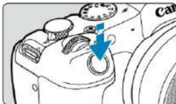
This activates autofocus and the automatic exposure system that sets the shutter speed and aperture value.
