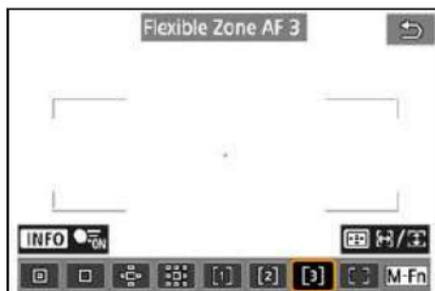
With Flexible Zone AF 1–3, you can freely set the size of the Zone AF frame (☑). Uses auto selection AF in Zone AF frames to cover a larger area than Expand AF area, which makes focusing easier than with 1-point AF/Expand AF area and effective for moving subjects.
