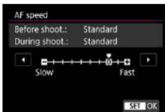
You can adjust the AF speed (focus transition speed) from the standard speed (0) to slow (one of seven levels) or fast (one of two levels) to obtain the desired effect for the movie creation.
