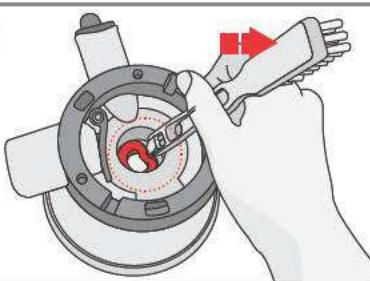
If the bowl packing at the bottom of the bowl is not fully inserted and is bent, set it into place with the rotating attractor of the cleaning brush.
