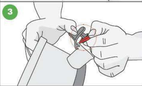
Set the packing to seal off completely. If not completely sealed, juice may leak.
