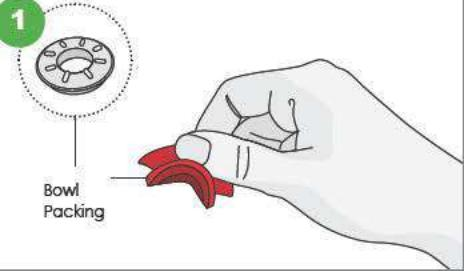
As shown to the left in the dotted circle, let the protrusion part on the bowl packing face upward and hold it, like pinching, with your thumb and index finger.
