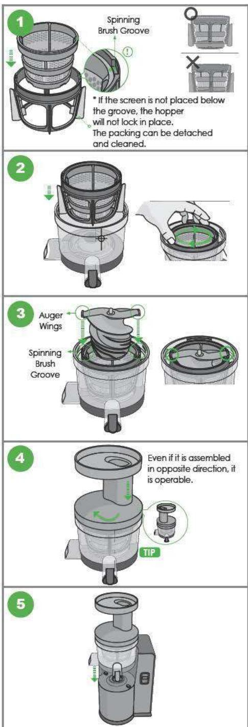
Assemble the screen. The top of the screen must sit below the grooves on the spinning brush, as shown in the picture. Otherwise, the chamber set will not close properly.
