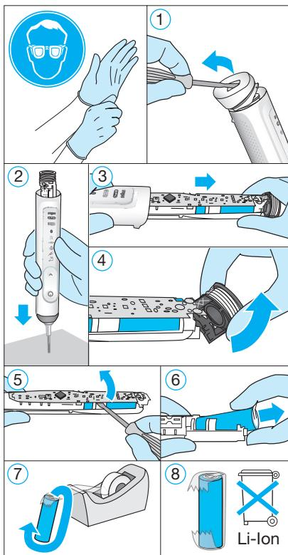
Open the handle as shown, remove the battery and dispose of it according to local environmental regulations.
