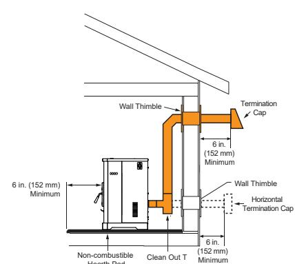
NOTE: In Canada when using a factory-built chimney it must be safety listed, Type UL103 HT (2100°F) CLASS "A" or conforming to CAN/ULC-S629M, STANDARD FOR 650°C FACTORY-BUILT CHIMNEYS.
