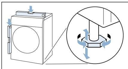
3. If necessary, turn the appliance feet to make sure it is level.
