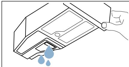
3. Push the condensation container back into the appliance until you feel it lock into place.
