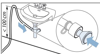
The connection point must be secured using a hose clamp (clamping range 12-22 mm).
