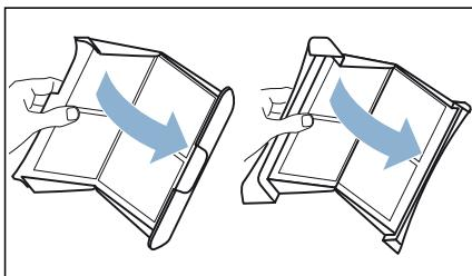
6. Remove all fluff from both parts of the filter.
