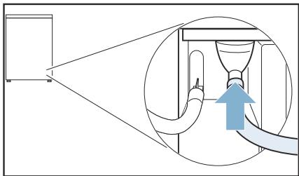
6. Secure the other end of the drain hose in place using the remaining accessories (depending on the connection type).
