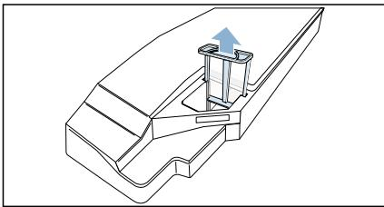
11. Place the filter into the recess on the condensation container.
