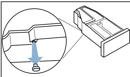
9. Turn the condensation container 180° again and insert the stopper into the recess in the top of the condensation container.
