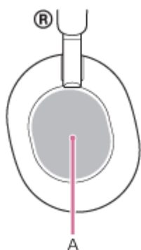
A: Touch sensor control panel
