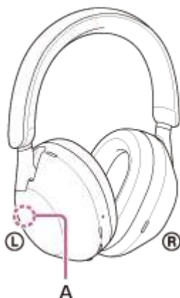
A: Location of the built-in antenna
