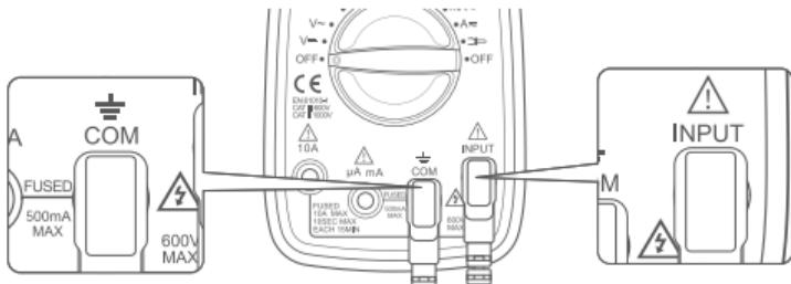
2. Operation: Turn the rotary switch to the " $\Omega$ " setting and choose the "Select" Button. Then, choose diode test mode, the " $\rightarrow$ " symbol will display on the LCD screen.
