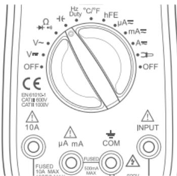
3. Connect Capacitance: Connect Capacitance, insert the red test lead into the positive pole and the black test lead into the negative pole.
