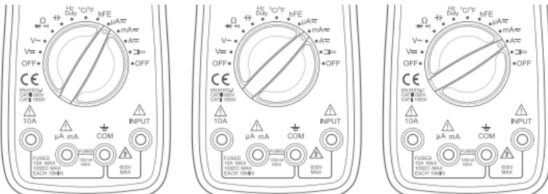
3. Choose current types: Press the "Select" Button to choose between a DC or AC current test.
