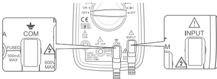
2. Choose functions: Turn the rotary switch to the "Hz/Duty" setting. Press the "Hz/Duty" Button to switch frequency measurement or duty ratio measurement.
