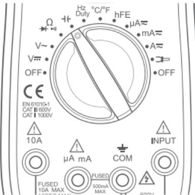
3. Connect Capacitance: Insert the Capacitance positive pole into the "INPUT" jack of the Multi-Function Socket and the negative pole into the "COM" jack of the Multi-Function Socket.
