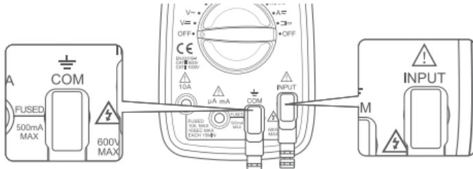
2. Turn the rotary switch to the  $\Omega$  setting, choose the "Select" Button. Then, select continuity Mode, the  $\bullet\bullet$  symbol will display on the screen.
