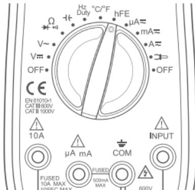
3. Measurement of Transistor: Identify whether the transistor is an NPN or PNP type, and identify emitter, base and collector terminals. Insert the terminals into the adapter transistor test socket.
