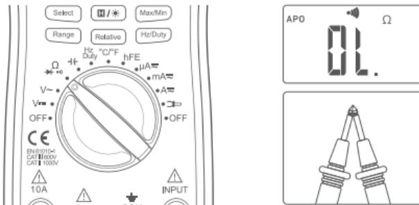
4. Connect load: Place the test leads at both ends of the resistance or load to be measured.
