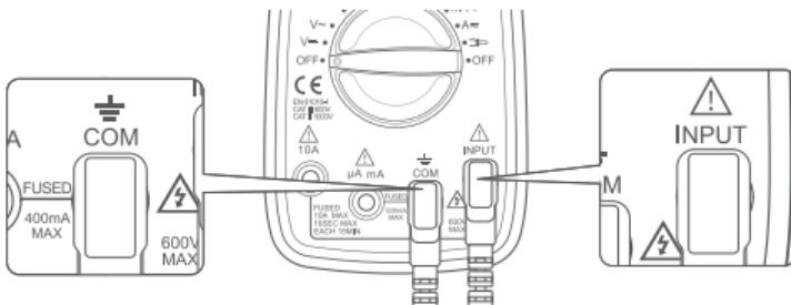
2. Choose functions: Turn the rotary switch to the "V~" or "V=" setting according to the measured voltage.
