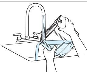
**4.** Pour out dirty water. Rinse tank to remove any debris.
