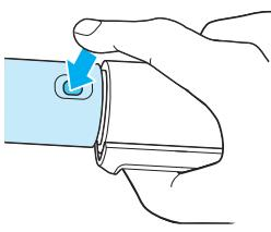
**2.** To disconnect tools, push down on button above hose grip and pull straight off. (Do NOT twist tool to remove it.)
