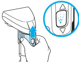
**4.** Slide tool lever up to ensure tool is in SPRAY mode. Follow cleaning steps on pg 4.
