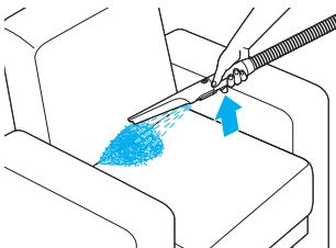
**1.** While holding tool above the stained area, press and hold the trigger to spray solution.
