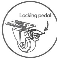
Press the pedal down to engage the lock. To unlock, lift the pedal up.
