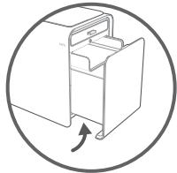
Open the bottom drawer, reach into the bottom to locate the front wheels.
