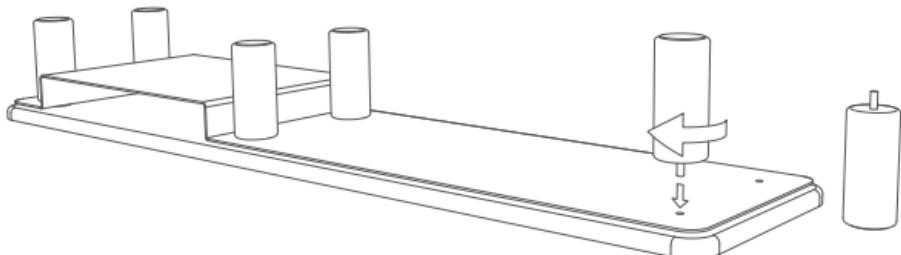
Tighten the wooden legs with bolt clockwise into the shelf.
