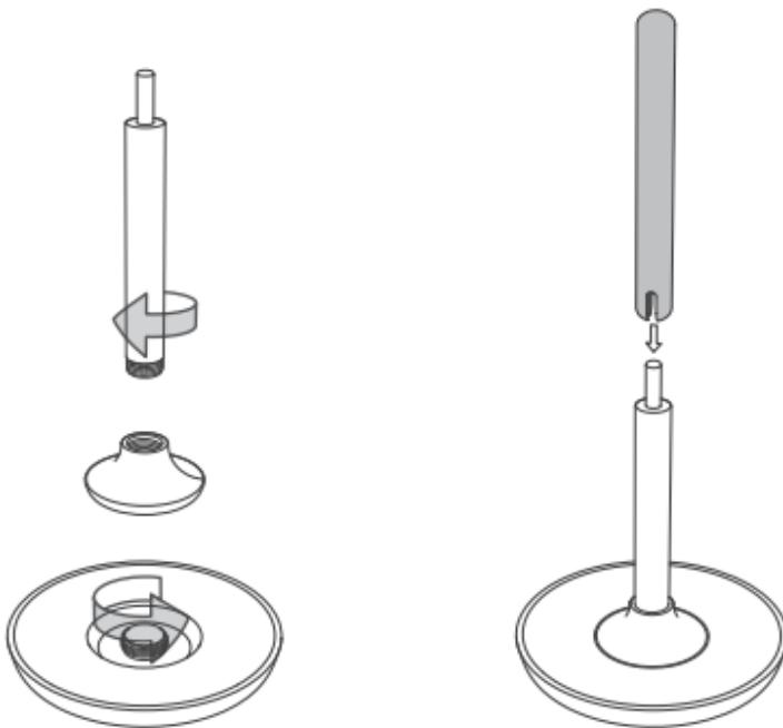
The inner pillar should be screwed onto the mount base clockwise, the mount base can be screwed onto the weight base clockwise.
