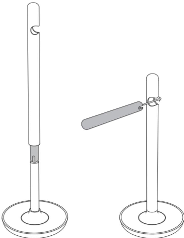
Insert the wooden stick through the horizontal notch on the outer pillar to hang the headset on the stick.
