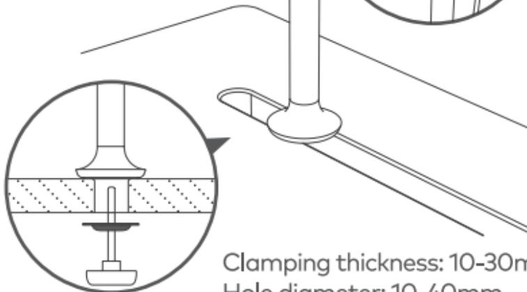
Clamping thickness: 10-30mm
