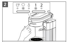
Turn On the Espresso Machine and toggle the Mode button to select Steam.
