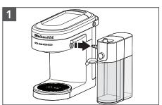
Press the Steam wand release button on Espresso Machine to release Milk Frother Attachment.
