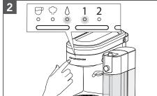
Turn On the Espresso Machine and toggle the Mode button to Water. Toggle the Dose button to 1 or 2 (1 for less water and 2 for more water).
