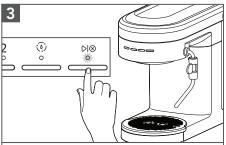
Angle the Steam wand towards the Drip tray or into a cup. Press ▶|⊗ button to start. Once water turns to steam, press ▶|⊗ button to stop.
