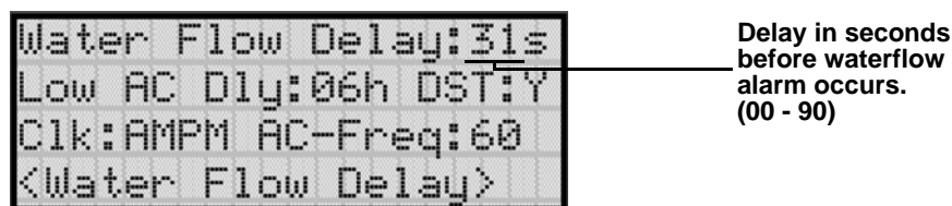
Figure 7-20 Water Flow Delay Programming Screen
