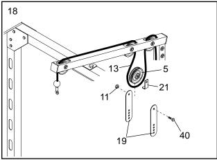
19. Route the indicated end of the Low Cable (8) around a Pulley (5). Attach the Pulley to the bracket on the Base Crossbar (20) using an M10 x 45mm Bolt (40) and an M10 Nylon Locknut (11). Do not overtighten the Nylon Locknut; the Pulley must be able to turn freely.
