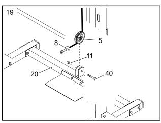
20. Route the Low Cable (8) around a Pulley (5) as shown. Hold a Cable Trap (21) against the Pulley and attach the Pulley and Cable Trap to the lowest holes in the two Pulley Plates (19) using an M10 x 45mm Bolt (40) and an M10 Nylon Locknut (11). Make sure the Cable Trap holds the Low Cable in the groove of the Pulley. Do not overtighten the Nylon Locknut; the Pulley must be able to turn freely.
