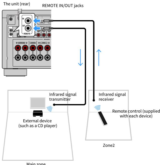
An infrared signal transmitter is not required if you are using Yamaha products that support remote connections, as the unit does. You can transmit remote control signals by connecting the REMOTE IN/OUT jacks with monaural mini-jack cables and an infrared signal receiver.
