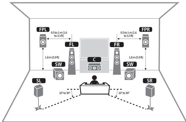
■ For layout with front presence speakers in Overhead position
