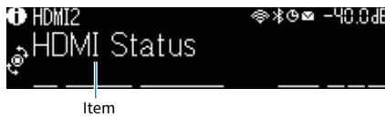
Push SELECT/ENTER on the front panel to switch the front display to the info select mode. And rotate SELECT/ENTER to select between the various items. The additional information is displayed under the item.
