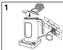
1. Add water to below the maximum water level line, plug in the power supply.
