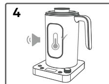
4. After reaching the set temperature, the machine will beep and finish its work.
