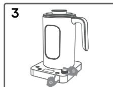
3. Rotate the knob to set the temperature or click "Custom temperature", then press "power button" to start heating.
