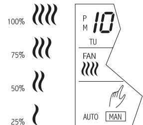
If you have programmed the heating control to ON/OFF to control a fan equipped system, the display will show the fan indicator and 100% when the heating system will turn ON and 0% when it will turn OFF. In this case, the temperature regulation will be ±0.5 °C around the setpoint.
