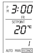
The ECONO mode has two (2) programs in which the day, the time and the setpoint has to be programmed. For instance, this operating mode can be used for a cottage installation where the user goes only on weekends.
