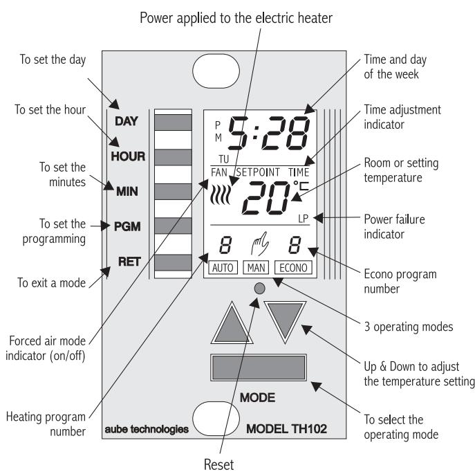
**NOTE:** To access the programmable keyboard, remove the cover by placing your fingers to the right side of the thermostat and pull toward you.
