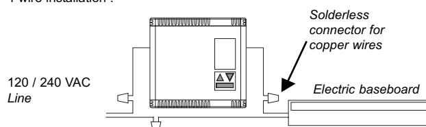
Push the excess wire back into the electrical box to prevent interference with the thermostat. Secure the thermostat using the supplied screw. Once the thermostat is properly installed, return power to heating system.
