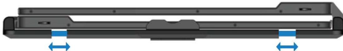
When folding the screens, pull the bracket out to the appropriate position, and fix the screen in the silicone of the bracket. Otherwise , forcibly closing will damage the screen.
