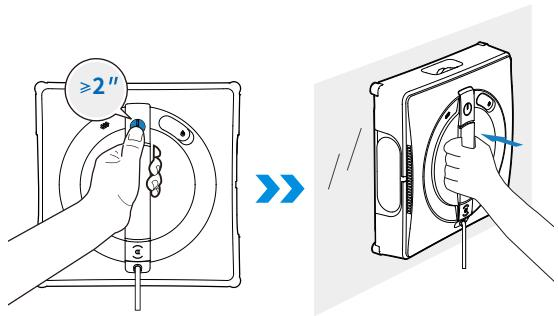
6. When cleaning is completed, WINBOT automatically returns to the Initial Spot and waits to be removed. At this point, long press START button for 2 seconds to stop the fan. Then, take WINBOT off according to voice prompts.
