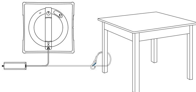
5. Long press START button for 2 seconds to start the fan. Place the bottom side of WINBOT (the side with Wiping Pad) against the window; WINBOT will auto-attach itself and start cleaning.
